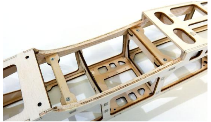
□ 24. Thoroughly sand the sides of the fuselage on the wing saddle area.
