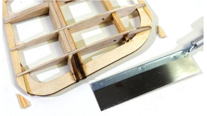
□ 67. Cut out L.E. and T.E. ends.
