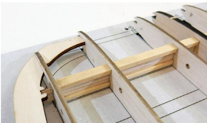
□ 25. Insert the shear web 32 between the front spars. Press the shear web 32 up to the slot in the wing tip 31. Don't glue!
