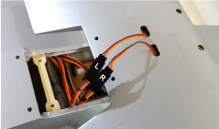
□ 5. Connect the aileron servo cables with servo leads from the receiver.
