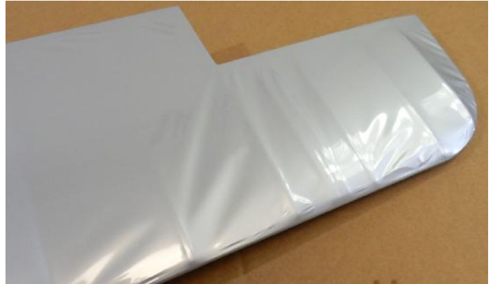
□ 14. Only iron the foil around the edges, do not shrink it or iron it to the ribs yet! It doesn't matter that the covering is corrugated now.
