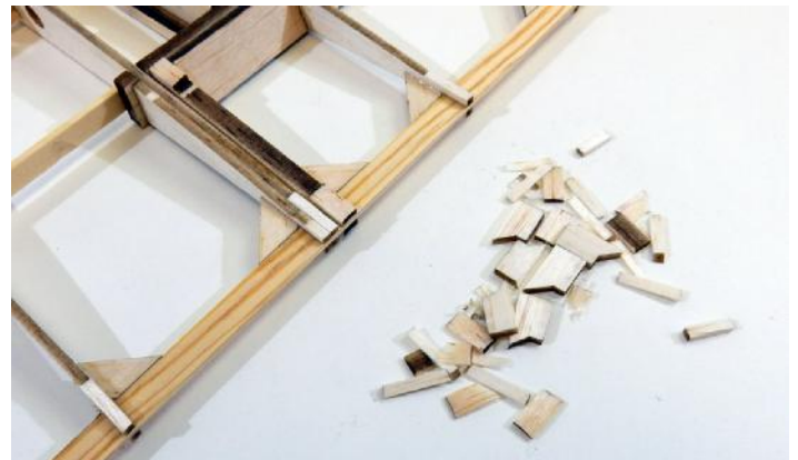
□ 61. Carefully cut off the supports from all ribs.
