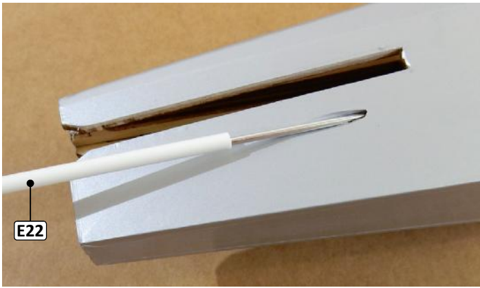
□ 32. Slide the tube E22 (length 350mm) onto the wire.
