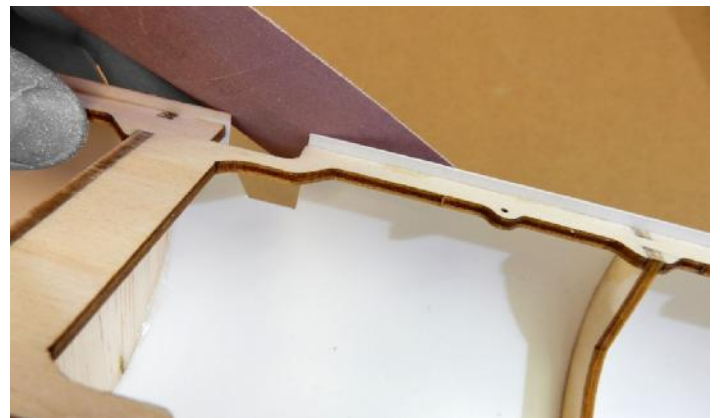
□ 53. Bevel all cover E1 edges with fine sandpaper (250-320).
