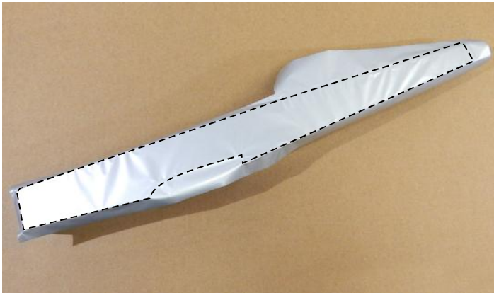
❑ 58. Continue by covering the left side of the fuselage. Again, iron on the edges first. Do not iron the covering on the upper rear part of the fuselage!
