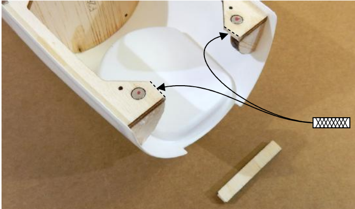
□ 32. Sand the cut edges with fine sandpaper (250-320).
