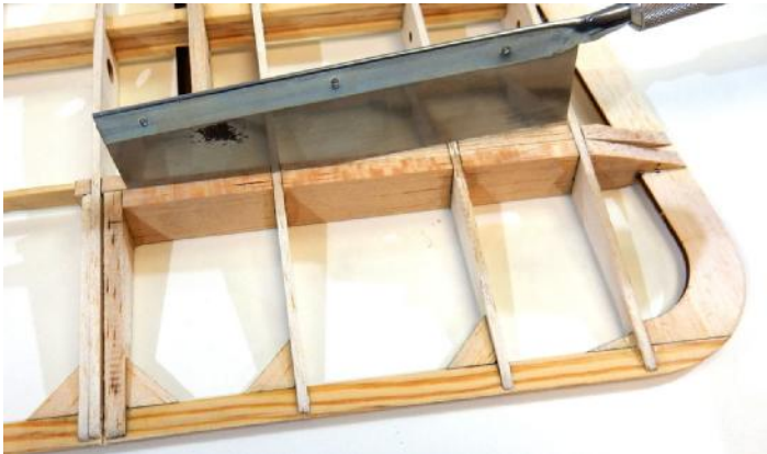
□ 92. Cut the ribs. Start as shown on the picture.
