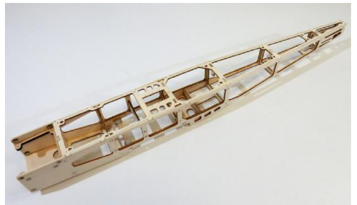
□ 26. The basic part of the fuselage is done. If you have been careful the upper side should be perfectly straight.
