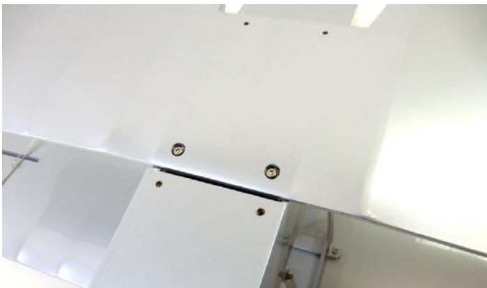
□ 7. Screw the bottom to the fuselage.
