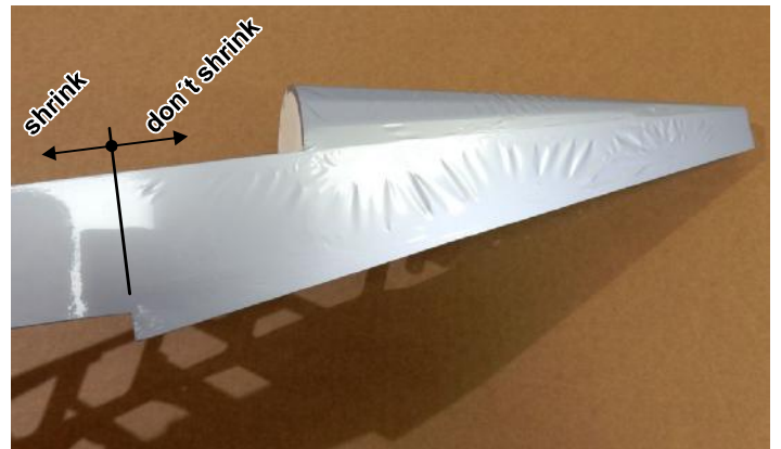
❑ 63. Iron the covering overlaps thoroughly. You can shrink the covering on the front of the fuselage, but do not shrink it on the back of fuselage now!
