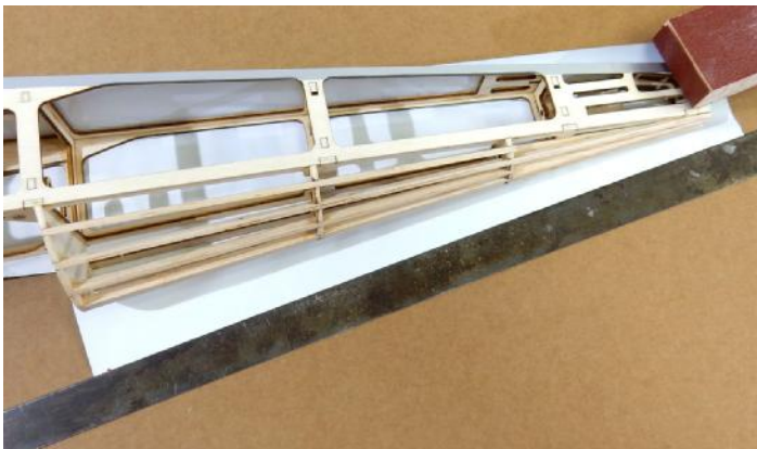
❑ 59. Trim the covering for the upper part of the fuselage according to the ruler so that edge of the covering ends at the balsa spar edge on the top (see the next picture).
