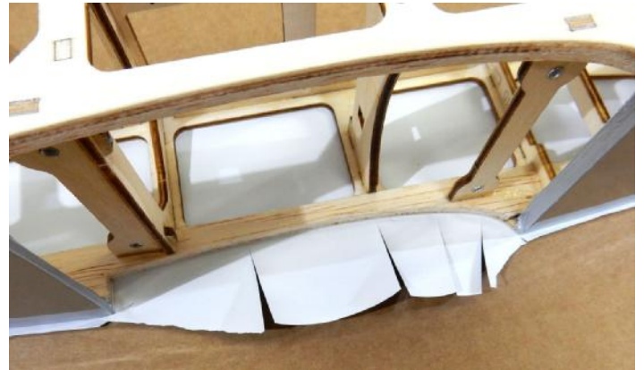
❑ 62. Cut the covering in the bottom wing saddle before ironing.
