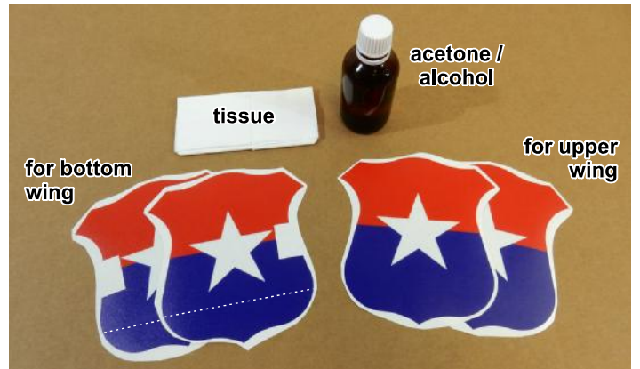
□ 12. Prepare wing stickers and clean the surface of the wings. Warning! The stickers for the bottom wing have cutouts for servos and are divided in the place of the aileron hinge.
