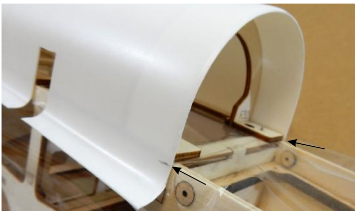
□ 41. The lines marked with pencil on both sides on the front of the cover should be placed similarly against the fuselage. Don't glue!
