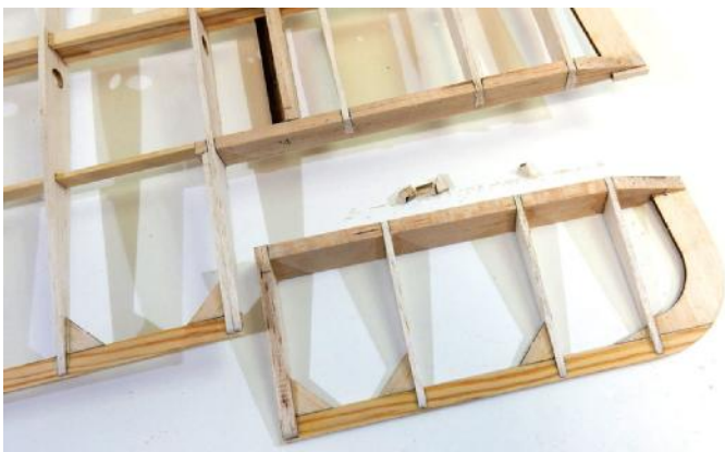
□ 93. Finally, cut off the wing tip 31. The aileron is separated.
