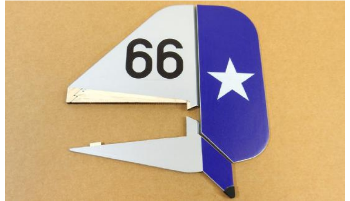
□ 11. The fin / rudder and tail skid are ready for final assembly.
