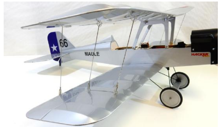
□ 10. Connect the wings with struts and ailerons with rods.
