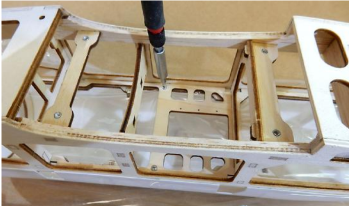
□ 48. Separate the cover E1 from the fuselage - remove the screws.
