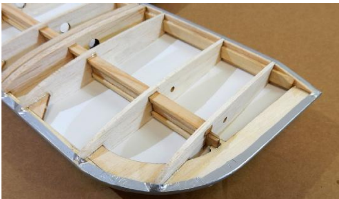
□ 12. With the iron set to a higher temperature, carefully iron the covering around the entire edges of the wing.
