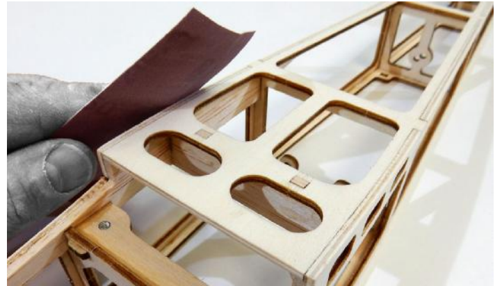
□ 25. Sand all "sharp" edges with fine sandpaper (250-320).
