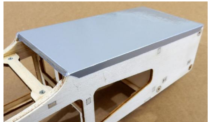
□ 55. Iron the overlaps thoroughly. You can iron this covering in the whole surface.
