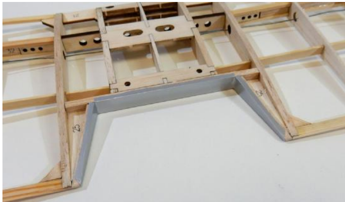
□ 4. Cover T.E. of the bottom center wing section.
