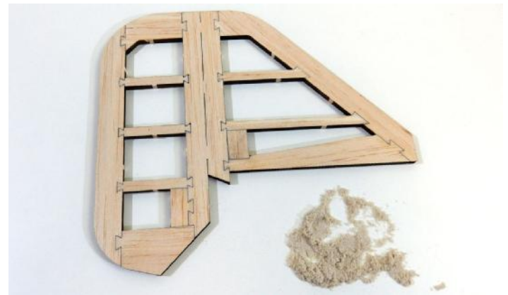
□ 3. Flat sand the stab/elevator assembly on both sides. We recommend using a respirator when sanding.
