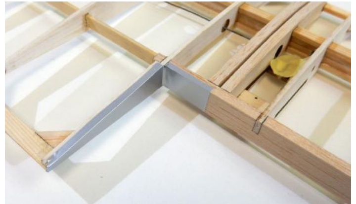
□ 6. Cover the inner corners at the ailerons.
