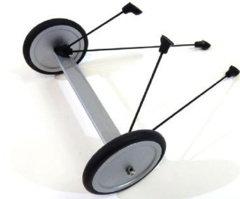
□ 8. Assemble the landing gear. Tighten the screws in the wheel stoppers E20 thoroughly.
