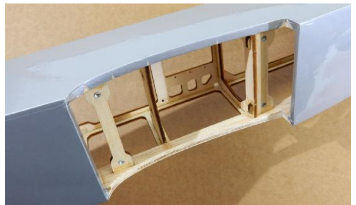
❑ 64. Iron the covering over the edges of the lower wing saddle and trim the overlaps.
