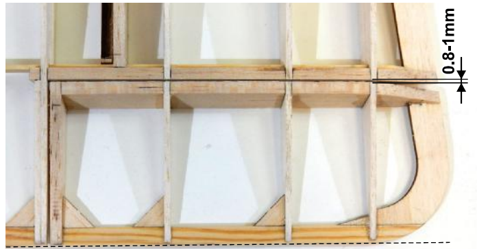
□ 95. Sand the aileron L.E. 15 to keep a gap of approx. 0.8-1mm between the wing and aileron. Wing T.E. must be aligned with aileron T.E.
