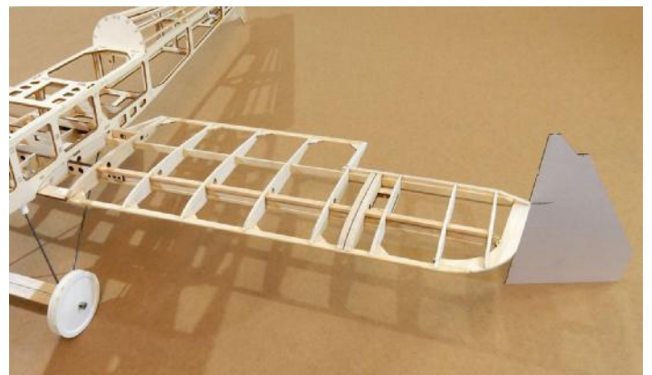
□ 13. Place the model on the landing gear and use the template to check that the wing tips on both sides have the same height from the table. Make a mark on the template with a pencil. You can change the geometry of the landing gear by moving the plastic parts on the wires.
