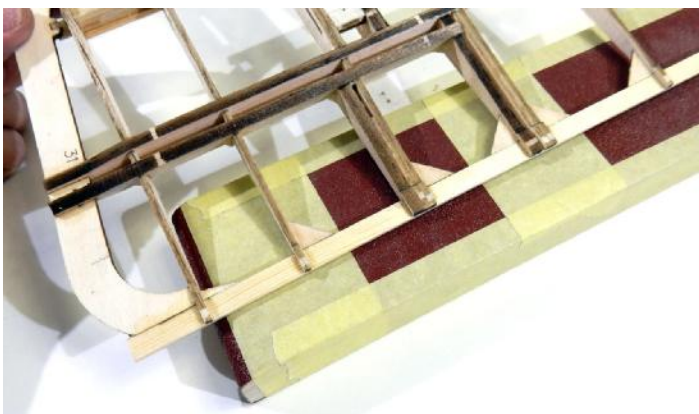
□ 64. Sand off the high spots on ribs around the T.E. Sand the ribs until follow the T.E.
