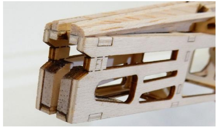
□ 69. Flat sand rear of the fuselage.
