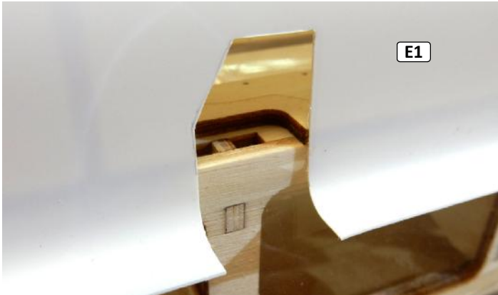
□ 39. Align the cover E1 with slots on cover frame (base sheet F27). Don't glue!
