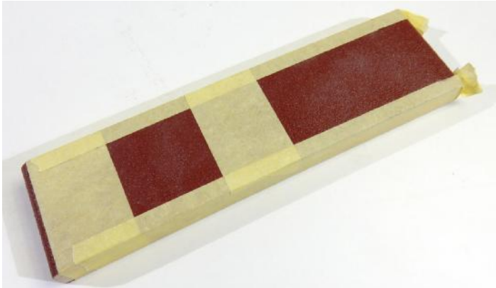
□ 63. Apply paper tape onto the sanding block. This will prevent you from sanding areas where you do not want to sand.
