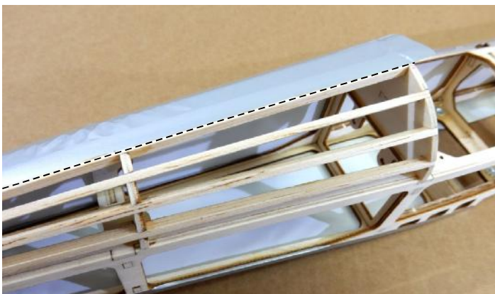
❑ 60. Iron the covering to the edge of top balsa spar.
