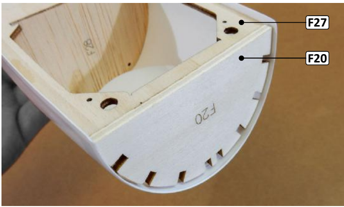
□ 55. Adjust the former F20 edge to follow the edge of the base sheet F27.
