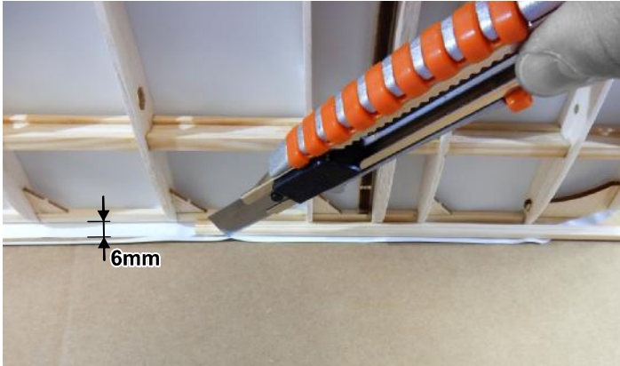
□ 10. Cut the covering along the L.E. with an overlap of approx. 6mm. You can use rest of spar 3x6mm as a spacer.
